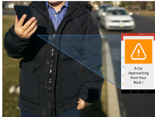
Fig. 1. Auto++ detects approaching cars using audio data recorded by smartphones. This capability can enable applications such as alerting distracted users (possibly through sounds or vibrations). Please note that the application logic such as alerting users is not part of Auto++.
