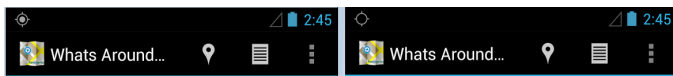
Fig. 1: One version of the existing Android location access disclosure (Google Nexus 4 with Android 4.2.2). On the top left corner, the symbol gets filled and unfilled when the foreground app uses GPS localization. Different versions and vendors of the Android platform have used different kind of symbols, for example, a blinking satellite on the right side of the notification bar. Our research (as anticipated) indicates that this is not an effective disclosure.
